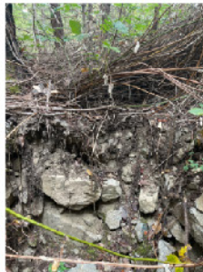
6 Excavation pit. (done by others). Consisting of cobbles, gravels and sands.
