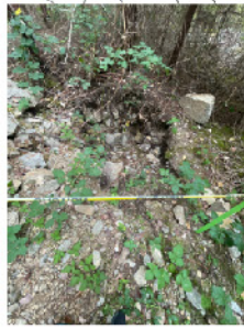
6 Excavation pit. (done by others). Consisting of cobbles, gravels and sands.
