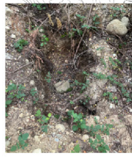
5 Excavation pit (done by others) consisting of cobbles, gravels and sands.
