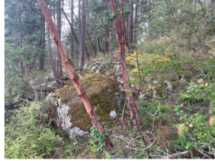
11 As per Golder (1983): "Slope treatment is needed." GES concurs with this recommendation. More broken rocks, indicative of previous rock sliding.
