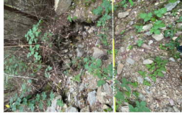
6 Excavation pit. (done by others). Consisting of cobbles, gravels and sands.
