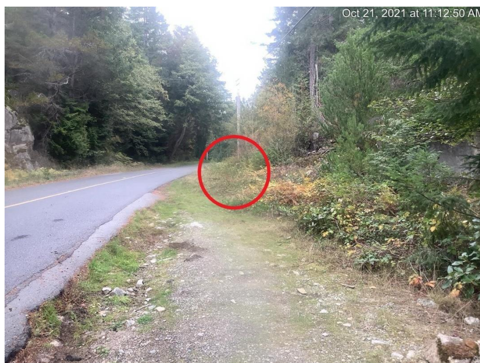
Photo 14. Looking north at the same watercourse along Truman Road overgrown with vegetation. The watercourse originates directly beside the road (orange circle) formed by runoff, then diverts away from the road and into the property near the trail entrance.
